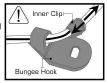
**Hint:** Before reattaching the Inner Clip/ Bungee Hook, tie a slip knot under slight tension at the lower bungee pulley. This will keep the bungee under tension while reassembling the Bungee Hook.
