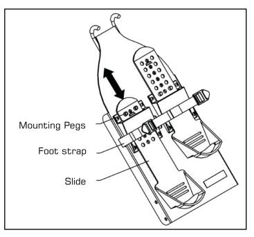
WARNING: Never operate this Rower without feet properly secured in Footstraps, or without the sliding portion of the Slider Footplate locked into position!
