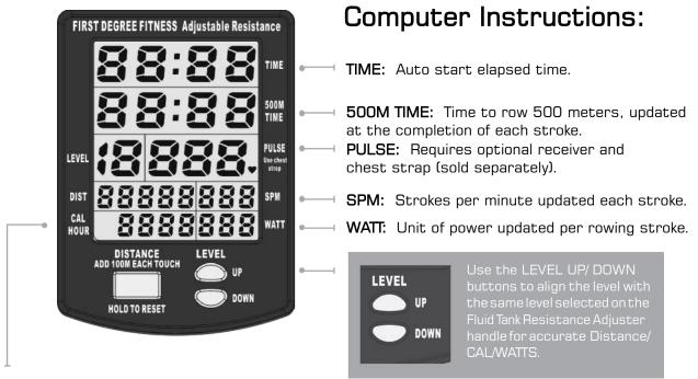
**CAL HOUR:** Calories burned per hour at the current Watts. Shows total calories burned when exercise is stopped.
